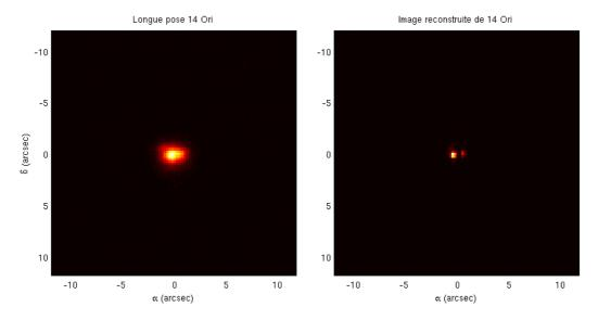
Image reconstruction test of the binary star system 14 Ori (H=4.6 magnitude), recorded in the astronomical H band (1.625 $\mu$ m) on October, 24 2014 at the Cassegrain focus of the 1 meter Omicron telescope of the C2PU facility (Observatoire de la Côte d'Azur). (left) Stack of 3000 co-added, 15ms exposure frames. (right) Reconstructed object from the 3000 short-exposure images.
