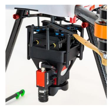
Easy integration on a UAS together with the Cubert mounting kit, compatible with any drone
