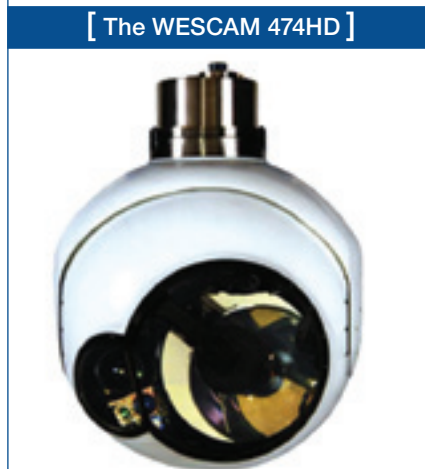
The WESCAM 474HD is a large shared-aperture SWIR and MWIR system recently developed at L-3 Communications / Wescam-Sonoma. It uses a combination of reflective and refractive optics. An 11-in. shared-aperture front end supports both spectral bands. The spectral light paths are split, and more traditional zooming (multiple field-of-view) refractive optics complete the imaging system.
