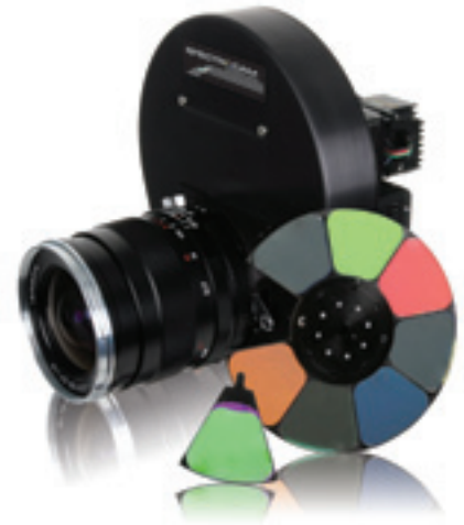
(Left) The infected lung tissue is imaged in eight bands in the visible and NIR with the SpectroCam MSI system and a standard light microscope. (Right) The SpectroCam has an internal eight-filter assembly, the wavelengths of which are custom defined by the user between 350 and 1,000 nm; end users can change filters in about one minute.
